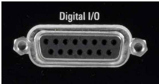
Digital I/O port on rear panel
