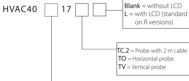
**Blank** = 0...20 mA / 4...20 mA active current analog output
