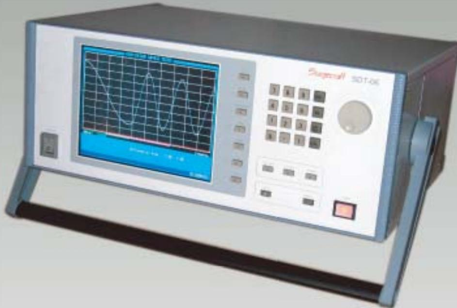
10-bit A/C Converter is adopted. High resolution provides extremely precise testing.
